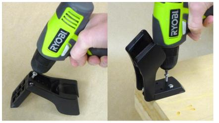
Secure the base to the holder using the (2) #10 x ¾" screws provided.
